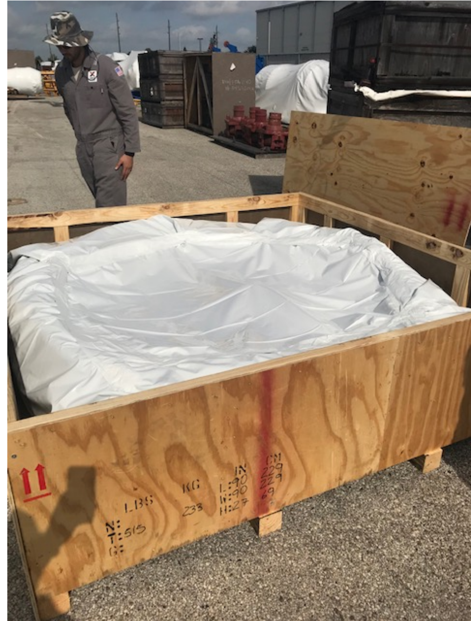
Fold and secure (tape, etc.) the top sheet to the bag to ensure it will remain in place.
