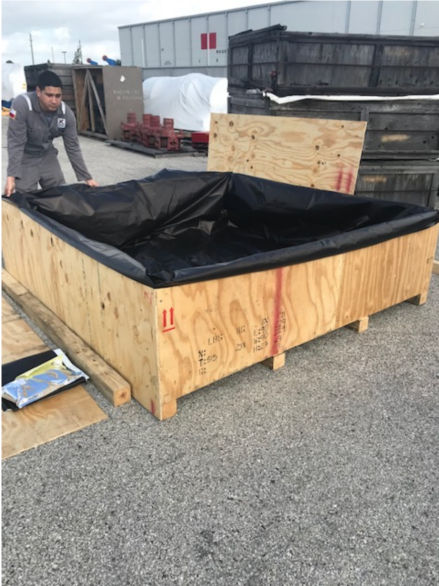
Open the Intercept Bag and place it flat on the bottom of the crate so that the dark brown side of the Intercept will be facing the part, as above.
